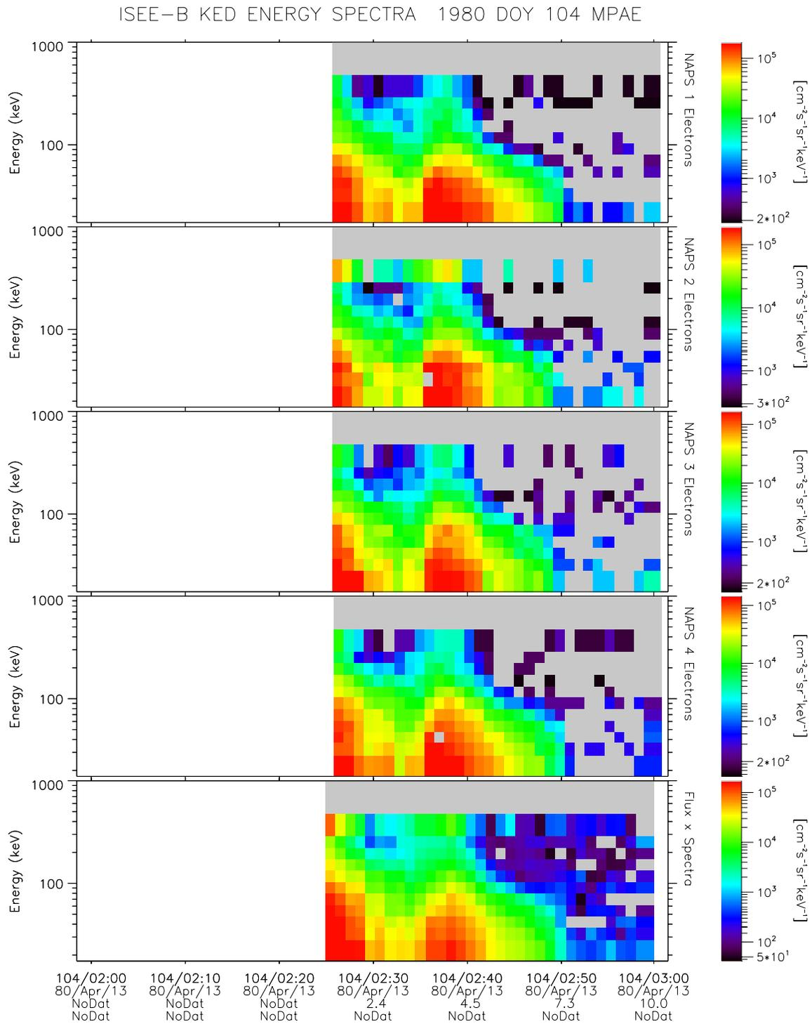
**Figure 8.7.** ISEE Example of four original dynamic energy spectra and the averaged spectrum. The first four plots show the data from the four NAPS sensors, the fifth plot shows the averaged spectrum adjusted to the total flux.
