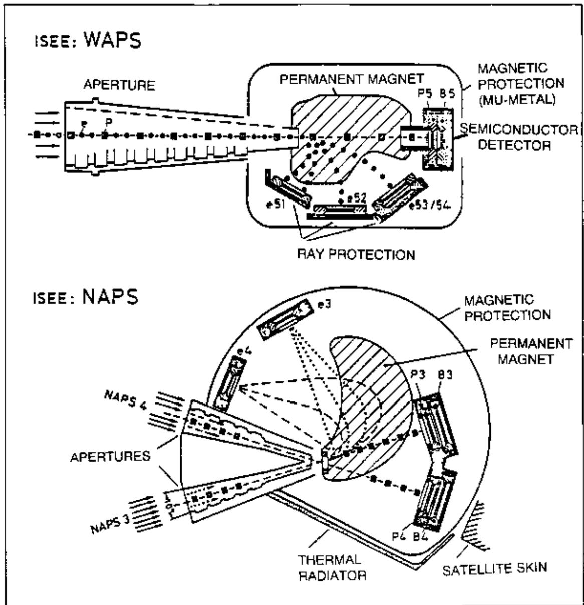
**Figure 8.2.** Cross section through the WAPS and the NAPS magnetic spectrometers. WAPS uses an inhomogeneous magnetic field to deflect electrons, NAPS a homogeneous magnetic field. Ions above the threshold energy of the instruments pass through the fields practically unaffected.
